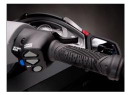
Yamaha's Electronic Throttle Control enhances your ride with several intelligent features. Cruise-Assist lets you set and maintain a specific speed while holding the throttle comfortably. No-Wake Mode allows for effortless navigation through controlled areas. Reverse Traction Control lets you manoeuvre smoothly by preventing over-revving when in reverse.
